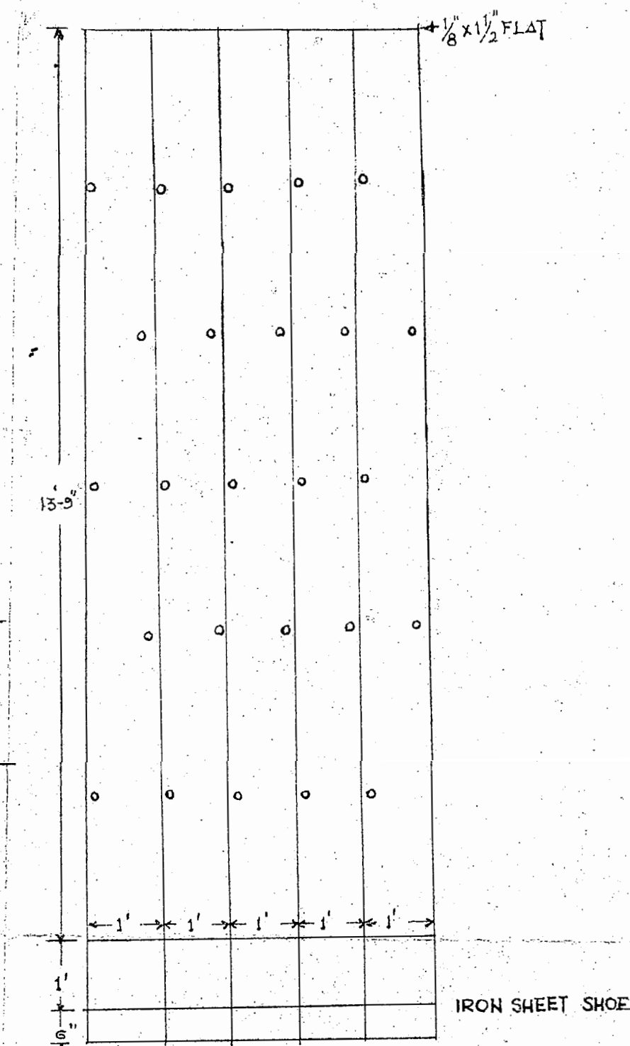
ELEVATION OF D/S PILES SCALE: 1"=2'
